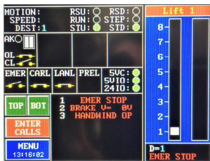
b. The Lift Menu “Lift Viewer” will show Hand-winding operation (as below)
