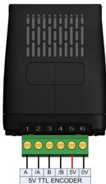
OPT-2-ENCOD-IN Connection Example – 5V TTL Encoder
