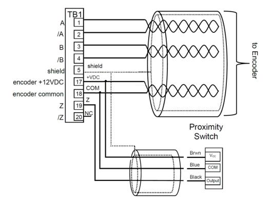
The wires are labelled, and should be connected into the terminals with the matching numbers in the **long** green terminal blocks.
