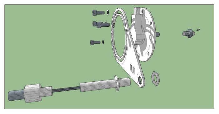
1. Fit the Rider wheel (05P00066-0622) to the encoder (Box 05P00057-0112) using the set screw (05P00302-6208).
