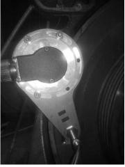
4. The target flag (43T02814-00XX based on which flag best fits) should be positioned on the sheave so that the short edge will face the proximity sensor. Use the alcohol wipe (05P00100-0064) to clean the surface, then fix target using the adhesive pad (05P00531-0025) Use the gap tool (43T02814-0020) to give correct distance
