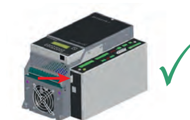
Memory card in the X-MMC card slot
