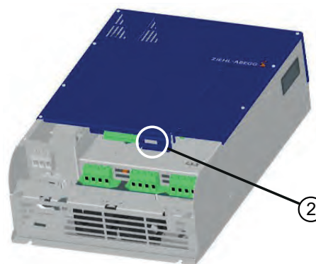
2 Position of card slot X-MMC on ZAdyn4C 040-074
