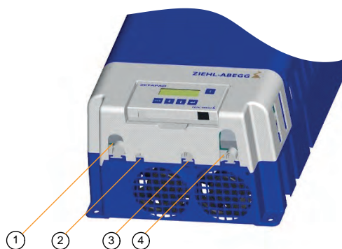
Cable layout front ZAdyn4C 011-032 1 Power line, X-OUT line 2 Protective earth connection 3 Brake resistor cable 4 Motor cable, cables X-DCP, X-IN, X-ENC8, X-CAN, X-MON, X-ENC8, X-STO
